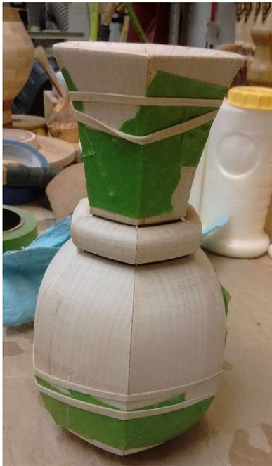
When the glue dries, you can use a disk or belt sander to flatten the mating surfaces, then glue the two halves together.
