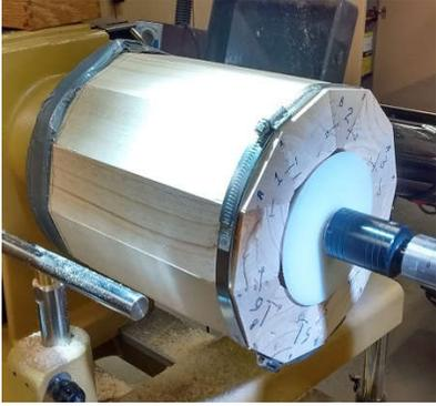
I used a cone on my live center to support the end of the assembled billets. Starting with the neck (tailstock end) begin forming the outside of the vase.
