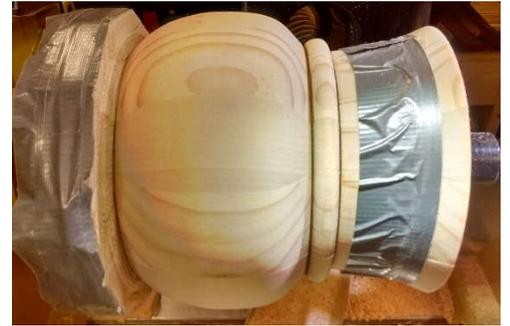
When you have the outside profile formed, wrap it tightly with either duct tape, filament tape, or shrink wrap. Make sure you wrap it tight ... you need all of the support you can get while hollowing the inside of the vessel.
