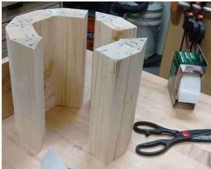
When you are satisfied with the miters, release the clamps and proceed to use double-face tape to assemble the billets, alternating mitered maple and square SPF. I used carpet tape, but any double-face tape should suffice.
